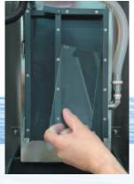
The unique sensing chamber design allows easy access to the controls and wetted components. The lamp/receiver unit is simply lifted and placed onto the convenient door rack. For any routine cleaning, the flow plate can be wiped in place or removed.
