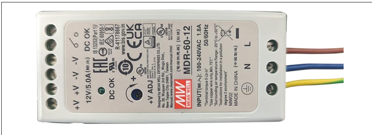
Figure 3 - Power Supply Unit Wiring to be done before use.
