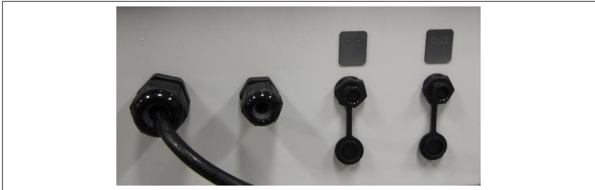
Figure 5 – 4-Pin female quick connect sockets for the sensors outlined by the red box.
